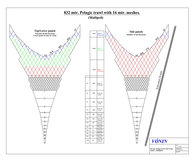
**Figure 1.** A drawing of the pelagic trawl Multpelt 832 m. This is a larger trawl, which is 832 m in perimeters and is designed for the mackerel investigations.
