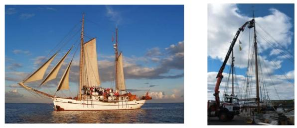
Figure 2. Left: Sailing vessel Donna Wood at sea. Note the long bow-sprit from which tags were attached using a hand-pole. Right: using a crane to mount VHF antennas on top of the 25m high foremast. Two downward looking video cameras were also placed near the antennae.
