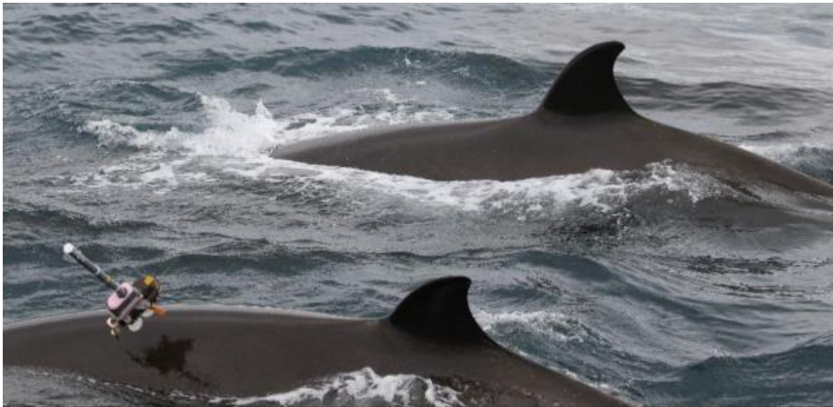
Deployment of the Mixed-Dtag on a northern bottlenose whale using the ARTS system.
