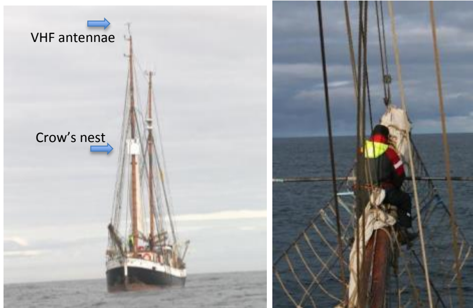
Figure 2. Left: Sailing vessel Donna Wood at sea. Arrows indicate the white observer crow's nest, and VHF antennae placed on the main mast. Four downward looking video cameras were placed near the crow's nest. The bow-sprit was used to attach tags using a hand-pole (right).
