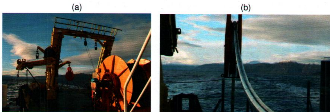
Figure 2: Pictures of measurement equipment: Winch with towed array aboard RV ELISABETH MANN BORGESE (a) and towed array before launching (b).
