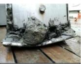
Figure 7.2c3 Image showing a rock and the damage it caused to the scoop.
