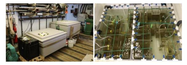
*Figure 7.4b Temperature controlled water baths and mesocosms containing sieved sediment and benthic invertebrates.*
