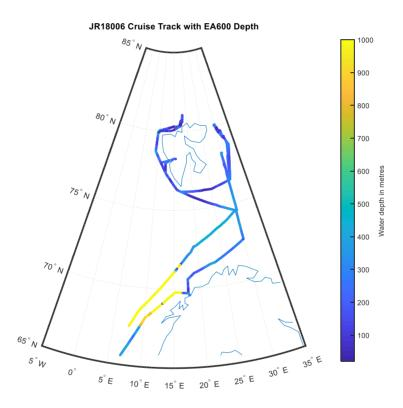
Figure 2.5c Cruise track showing EA600 echosounder bathymetry
