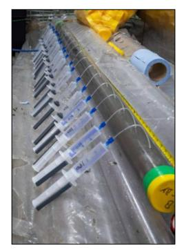
Figure 5.2a: Pore water extraction with Rhizone samplers and 30 mL syringes in the cold room. Photo: J. Faust
