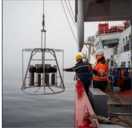
Figure 5.1b: Recovery of Megacorer (Photo: J.Faust)
