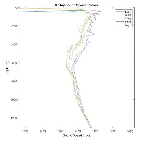
Figure 8: Sound Speed Manager comparison of all collected sound speed profiles from sub and XBT.
