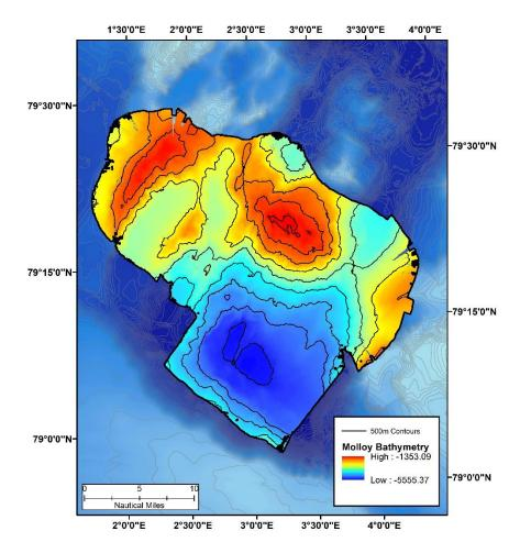
Figure 1: Molloy bathymetry collected with the Kongsberg EM 124 over GEBCO 2014 estimated bathymetry.
