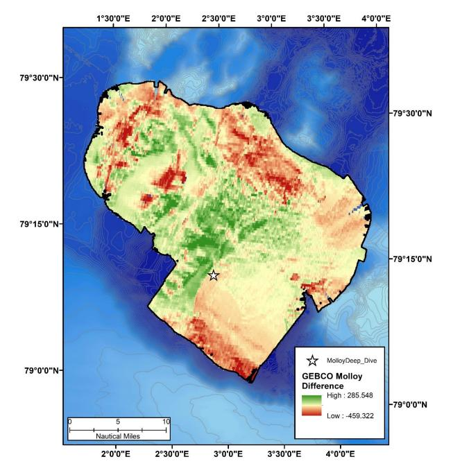
Figure 6: GEBCO 2019 bathymetric grid differenced with the Molloy data. Green indicated areas where Molloy is deeper than GEBCO estimates.
