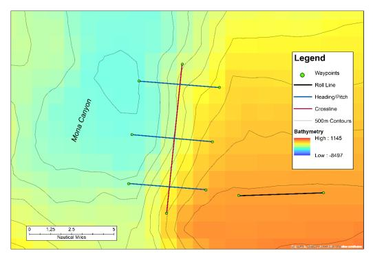
Figure 9: Sonar Acceptance Test (SAT) plan in the Mona Canyon offshore Puerto Rico and near the Puerto Rico Trench.
