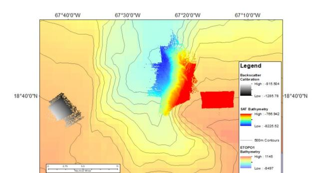
Figure 11: Backscatter calibration in relation to the SAT calibration site.
